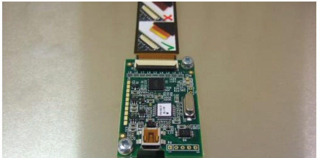
FIGURE 1 32 INPUT ZXY100/110° USB CONTROLLER FOR SMALL SENSOR SIZES
