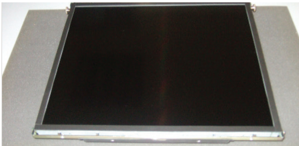
FIGURE 6 FOAM GASKET APPLIED TO LCD TO PROVIDE AIR GAP BETWEEN LCD AND SENSOR
