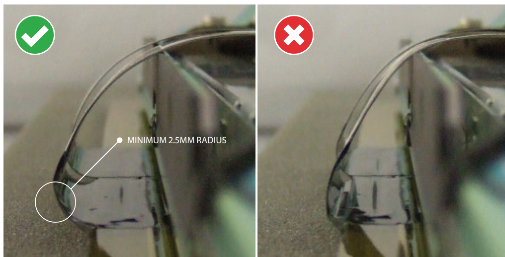
FIGURE 15 FLEXIBLE CABLE BENDING AT SENSOR EDGE
