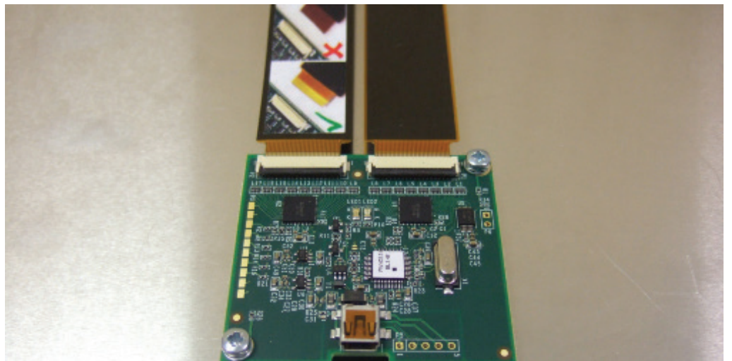
FIGURE 2 64 INPUT ZXY100/110° USB CONTROLLER FOR MEDIUM SENSOR SIZES
