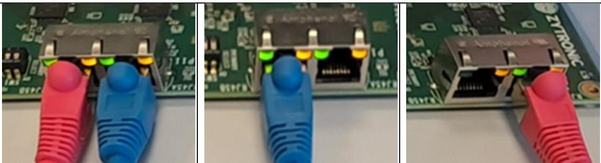
Cable from first secondary to second secondary is connected (blue). 2 green LEDs come on on the second secondary
