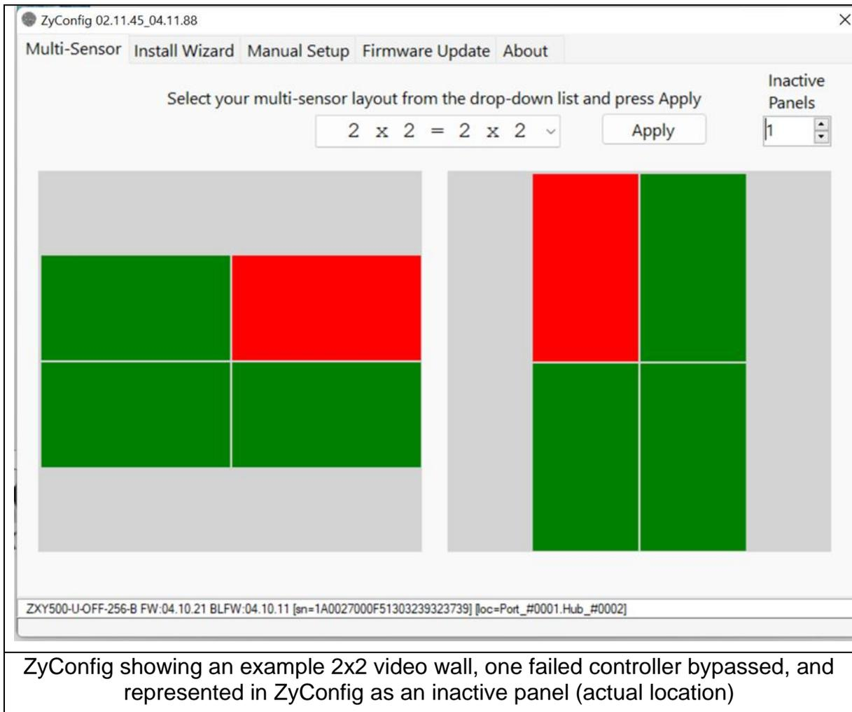
This video wall can now continue to be used, albeit with one panel not working, until a replacement part can be arranged and fitted.
