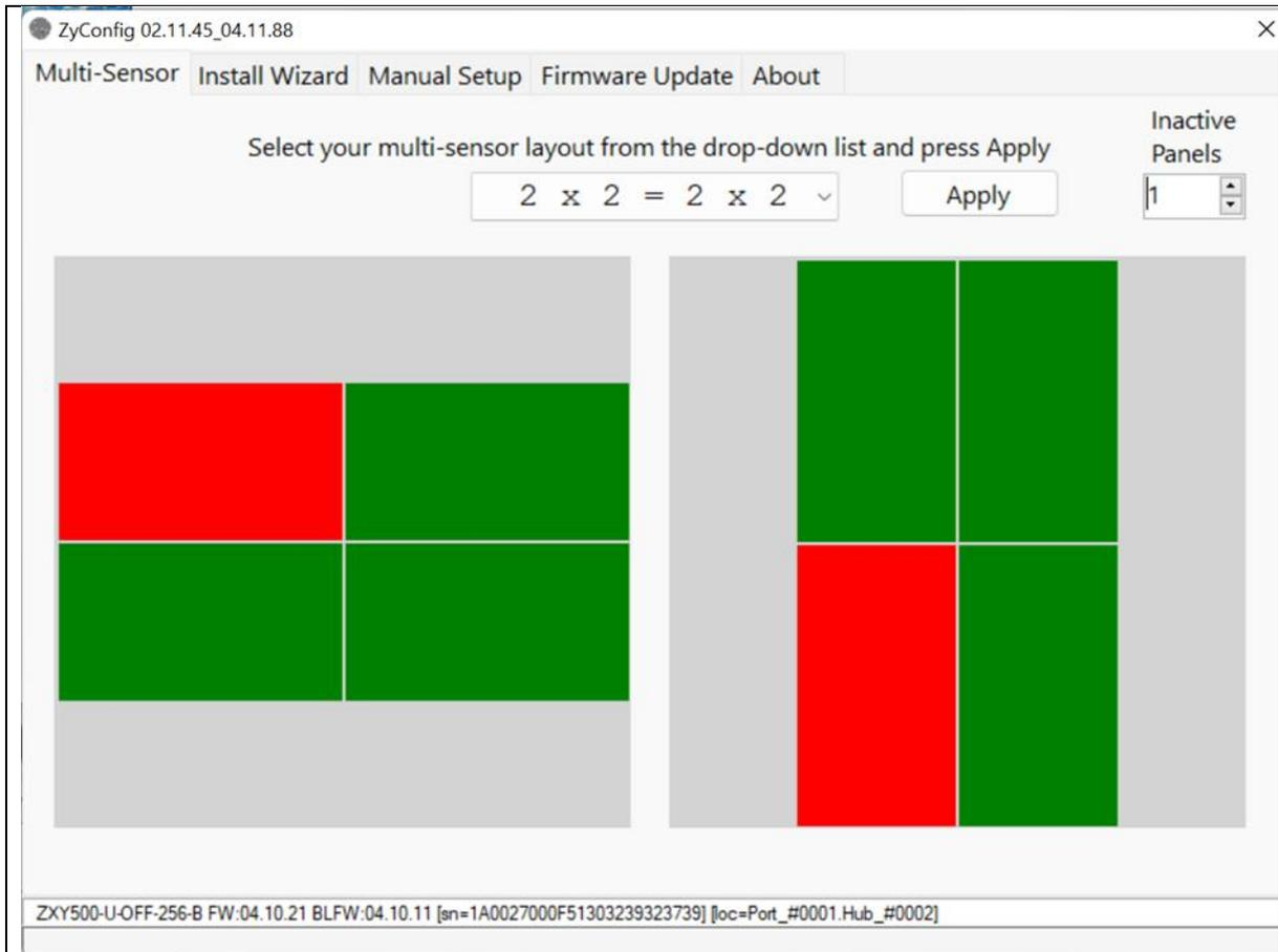
ZyConfig showing an example 2x2 video wall, one failed controller bypassed, and represented in ZyConfig as an inactive panel (default location)
