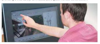
Zytronic's touch sensor technology is also readily scalable in size, allowing customers to use sensors ranging in size from 6 inches to 82 inches. Additional customisation can be provided, including printed borders, logos, etc.; non-rectangular shapes; shaped polished edges; and different glass substrate thicknesses from 1mm to 12mm.
