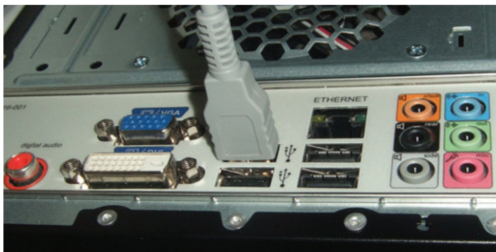
FIGURE 28 CONNECTING THE USB CABLE TO THE HOST PC
