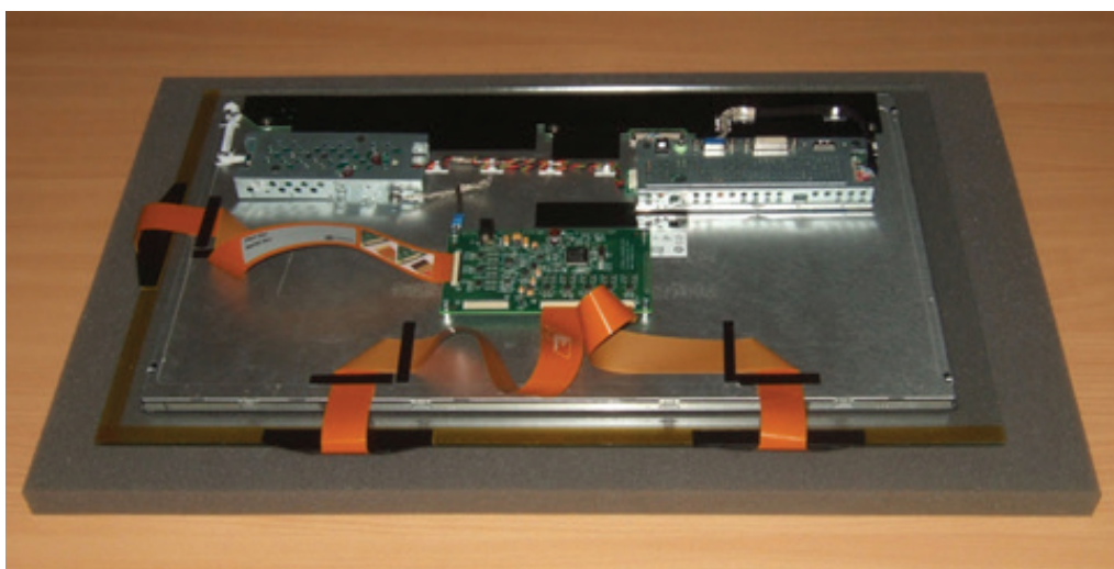
FIGURE 14 FLEXIBLE CABLES PLUGGED INTO THE CONTROLLER PCB
