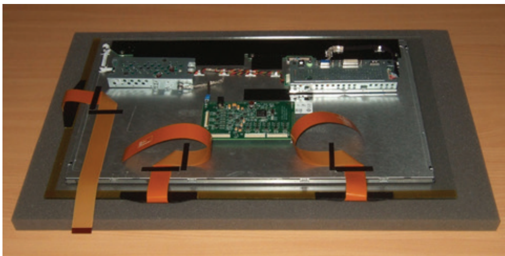
FIGURE 13 FLEXIBLE CABLES CAN BE CAREFULLY CREASED TO PRODUCE 90 DEGREE BENDS
