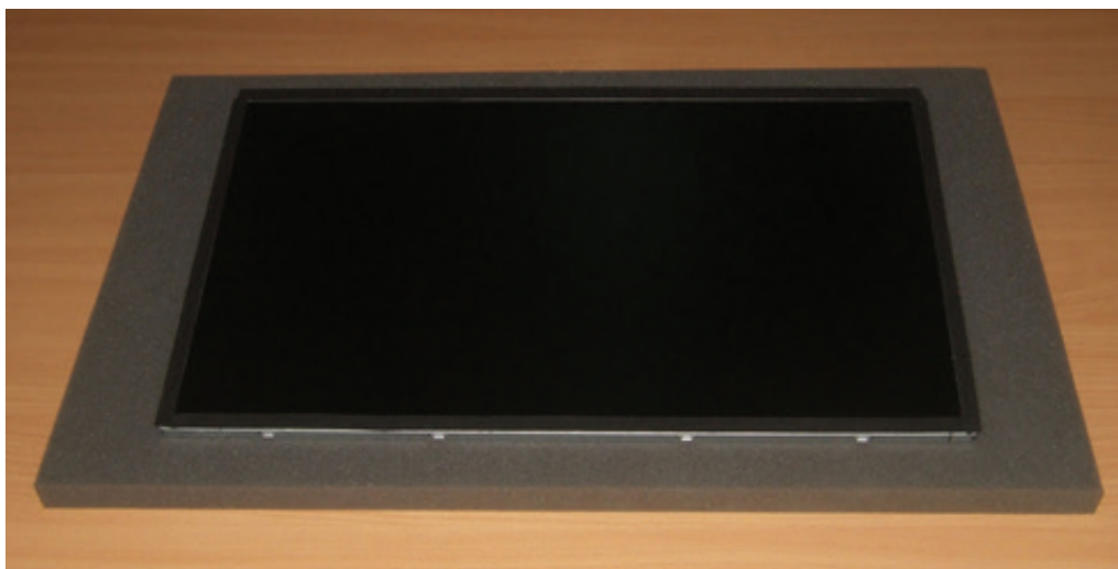
FIGURE 2 FOAM GASKET APPLIED TO LCD TO PROVIDE AIR GAP BETWEEN LCD AND SENSOR
