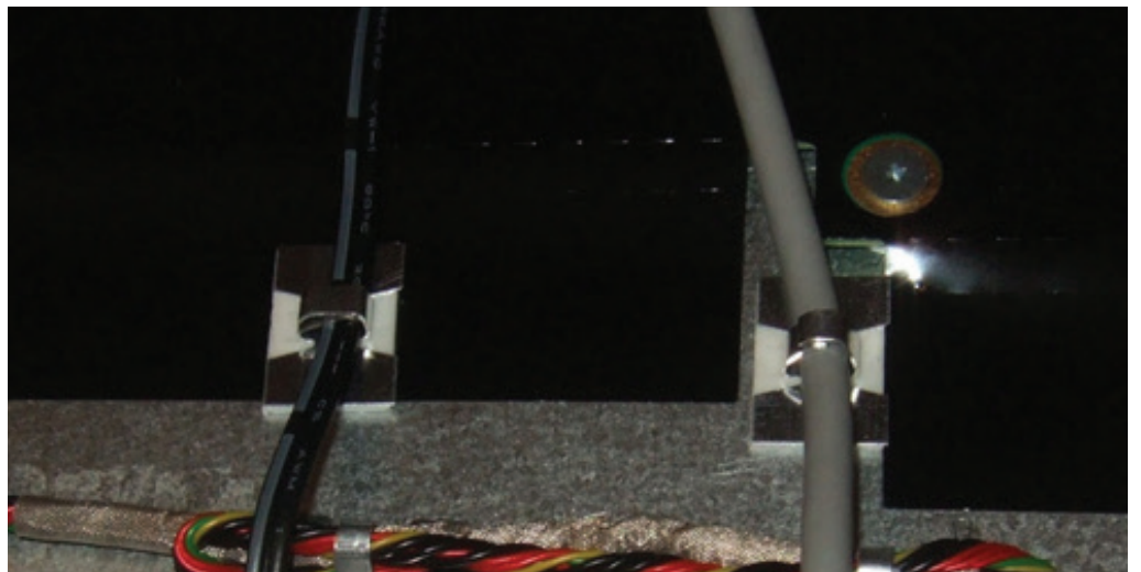
FIGURE 25 CABLE CLIPS HOLDING CABLES IN PLACE
