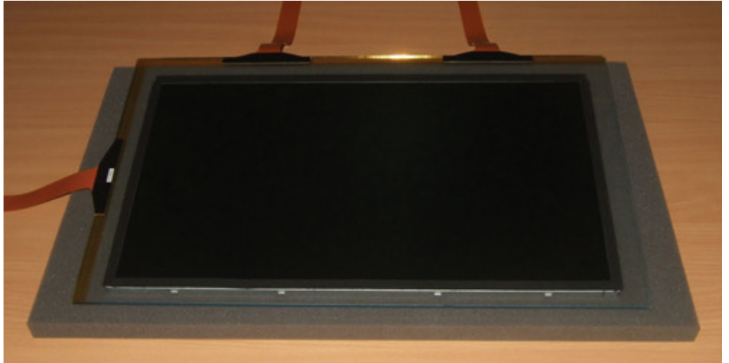
FIGURE 4 SENSOR MOUNTED ONTO LCD WITH GASKET
