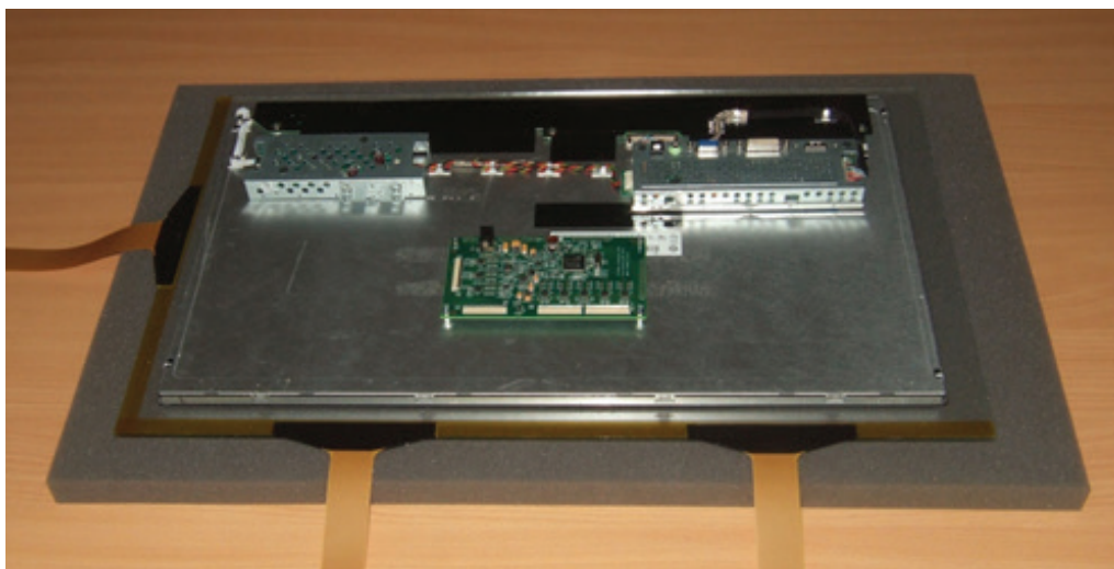
FIGURE 6 CONTROLLER POSITION ON REAR OF LCD
